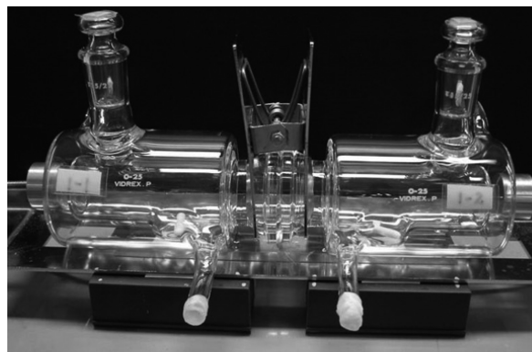
FIG. 1. Side-by-side membrane permeation cells for flat membranes used to measure free iodine. (PermcCell, VIDREX, KH-55, aperture diameter: 25 mm, membrane area: approx. 4.9 cm 2 , inside volume: approx. 55 mL)
