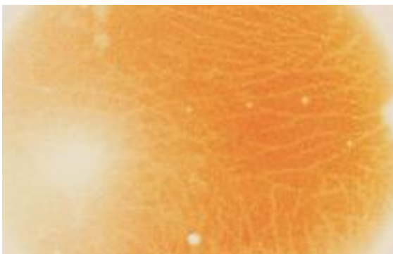
Snail Tracks, Stress Striae (Appendix 3 - Figure 4a)
